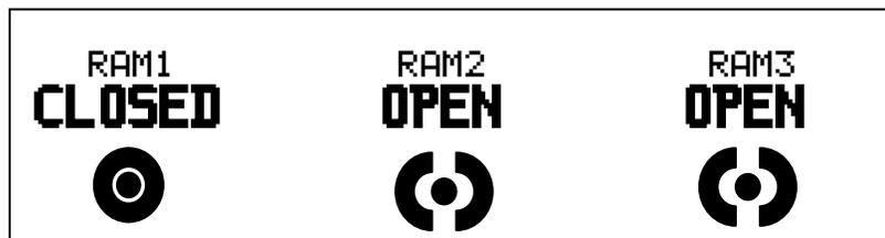
If you press the SELECT key, you will be taken to the secondary operation screen. On this screen BOP ram pair status, LED status and average ram pair temperature will be displayed.
